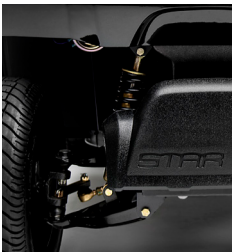
Independent suspension with double A-arms
