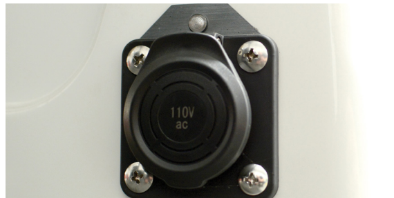
On-board charger and tri-color indicator
