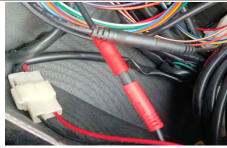
Connect the AUX cable and the head cable of the USB charger
